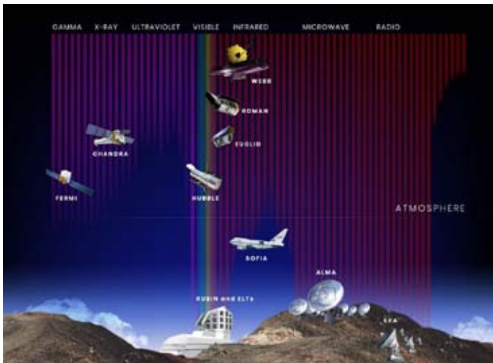
This illustration shows the wavelength sensitivity of a number of current and future space- and ground-based observatories, along with their position relative to the ground and to Earth's atmosphere. The wavelength bands are arranged from shortest (gamma rays) to longest (radio waves). The vertical color bars show the relative penetration of each band of light through Earth's atmosphere. Credit: NASA, STScI
